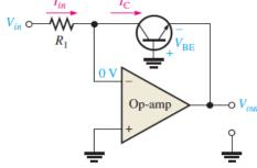
8. For the antilog amplifier in Figure, find the output voltage. Assume  $I_{EBO} = 40 \text{ nA}$ .
