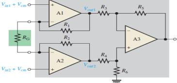
2. Calculate the voltage gain and determine the bandwidth using the graph in Figure. Modify the circuit for a gain of approximately 45.
