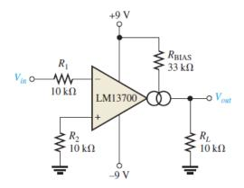
6. Determine the output voltage for the log amplifier in Figure. Assume  $I_R = 50$  nA.
